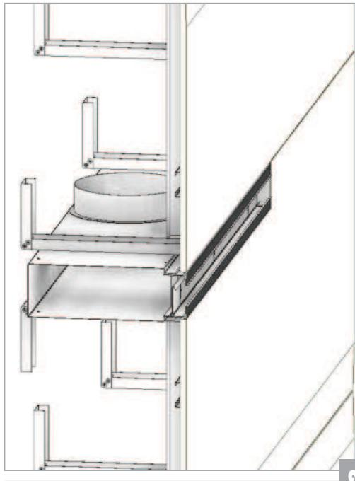
**5** Fix the diffuser to the false ceiling following the same steps as the assembly instructions "LOOK-SM ... (L), points 4 and 5"
