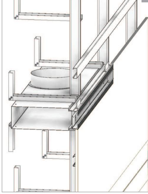
**4** Fix the diffuser to the false ceiling following the same steps as the assembly instructions "LOOK-SM ... (L), points 4 and 5"
