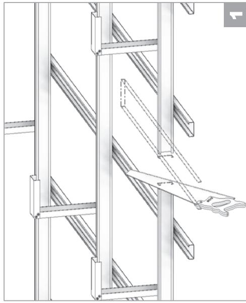
**1** Cut the ceiling structure or leave the space to enter the plenum box with the nominal sizes ( $A \times L$ ) mm.
